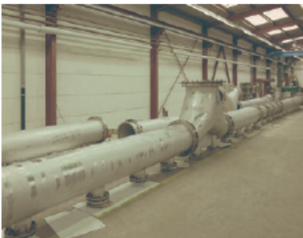
Rohrleitung aus Werkstoff Nr. 1.4435 \varnothing 711,2 x 6,0 mm/ Pre-manufactured pipe spool out of quality 1.4435 (316 L)
